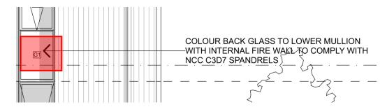
The detailed design stage design documents are required to show that any proposed spandrels including any support structure have an FRL of 60/60/60, that the openings protected by a horizontal spandrel are set back a minimum distance of 450mm and that they have a minimum depth of 1100mm.
