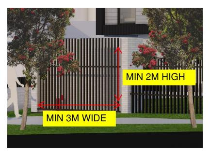
The fire hydrant booster location is not within sight of the main entrance of the building. As such will need to be addressed under a fire engineered performance solution.
